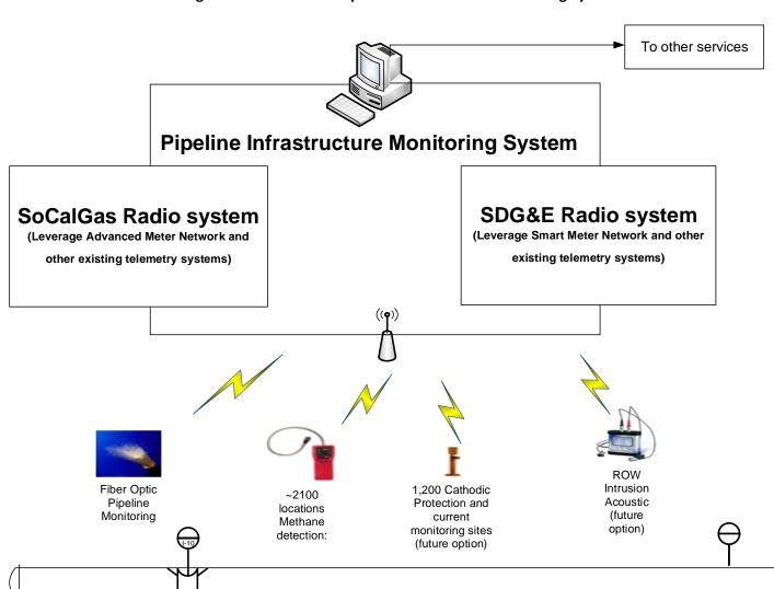
Figure 2 – Overview of Pipeline Infrastructure Monitoring System
