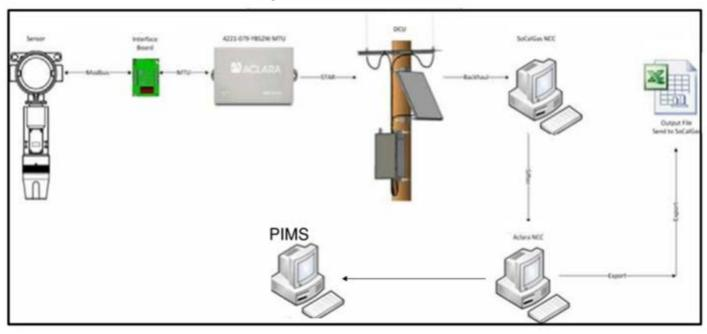
Figure 4: Methane Architecture
