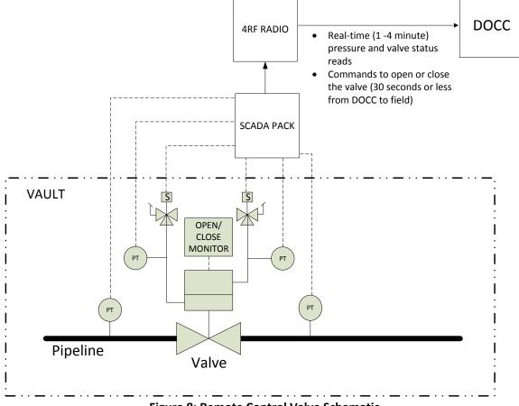
Figure 8: Remote Control Valve Schematic
