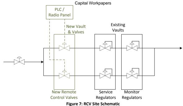
Figure 8 shows detail on how each RCV upstream of a regulator station will be equipped for remote operation and monitoring. Each valve will have an actuator for remote signal closure, along with telemetry points to monitor pressure on both sides of the valve. Outlet pressure and flow thru the regulator stations will also be monitored (not shown).
