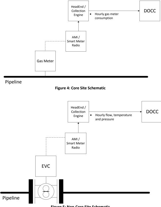
Figure 5: Non-Core Site Schematic
