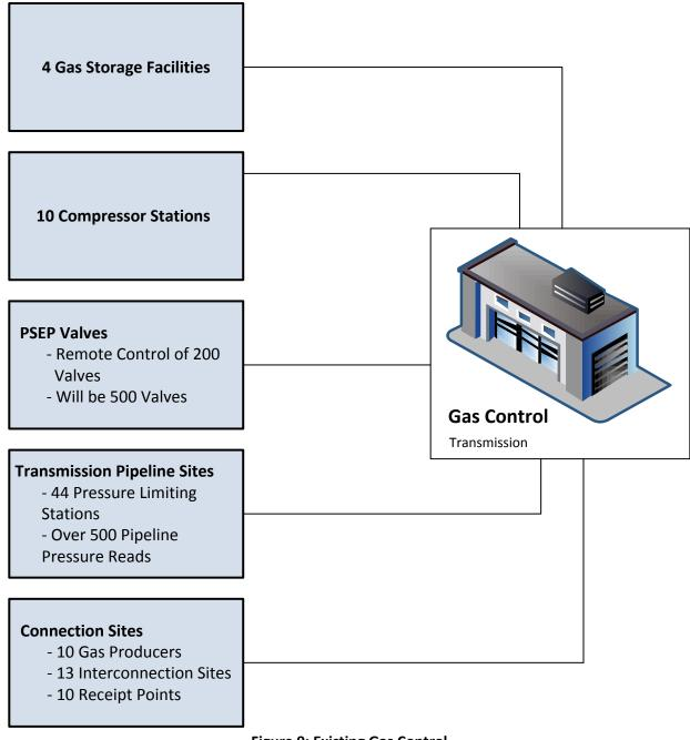
Figure 9: Existing Gas Control Data Architecture Capital Workpapers
